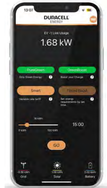
To change charging session mode whilst in another mode: Deselect current mode(s) Select desired new mode(s) Press 'Go'
